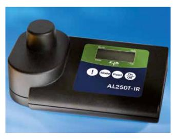
The compact AQUALYTIC® infrared turbidity measuring instruments AL255T-IR & AL250T-IR for fast and accurate on-site analysis. It is measured as provided in EN ISO 7027, the scattered light at an angle of 90  $^\circ.$
